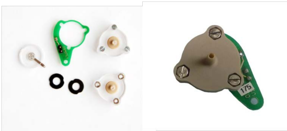
Figure 7: Closed evaluation package with fluidic and electric connectors (right) and its parts including the “Pump Core” (left). The fluidic connector has inner diameter 1.7 mm and outer 2.5 mm.
