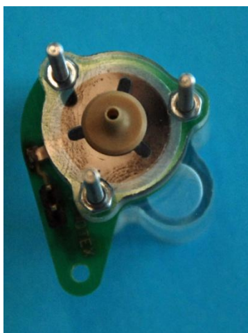
Figure 10: Open reservoir connector, bottom view. The fluidic connector has inner diameter 1.7 mm and outer 2.5 mm.
