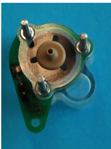
Figure 8: Open reservoir connector, bottom view. The fluidic connector has inner diameter 1.7 mm and outer 2.5 mm.
